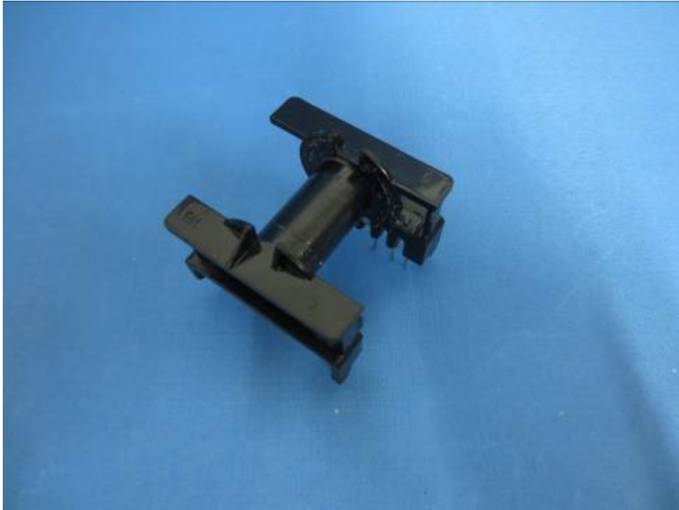
Bobbin of the transformer on control PCB (TA1)
