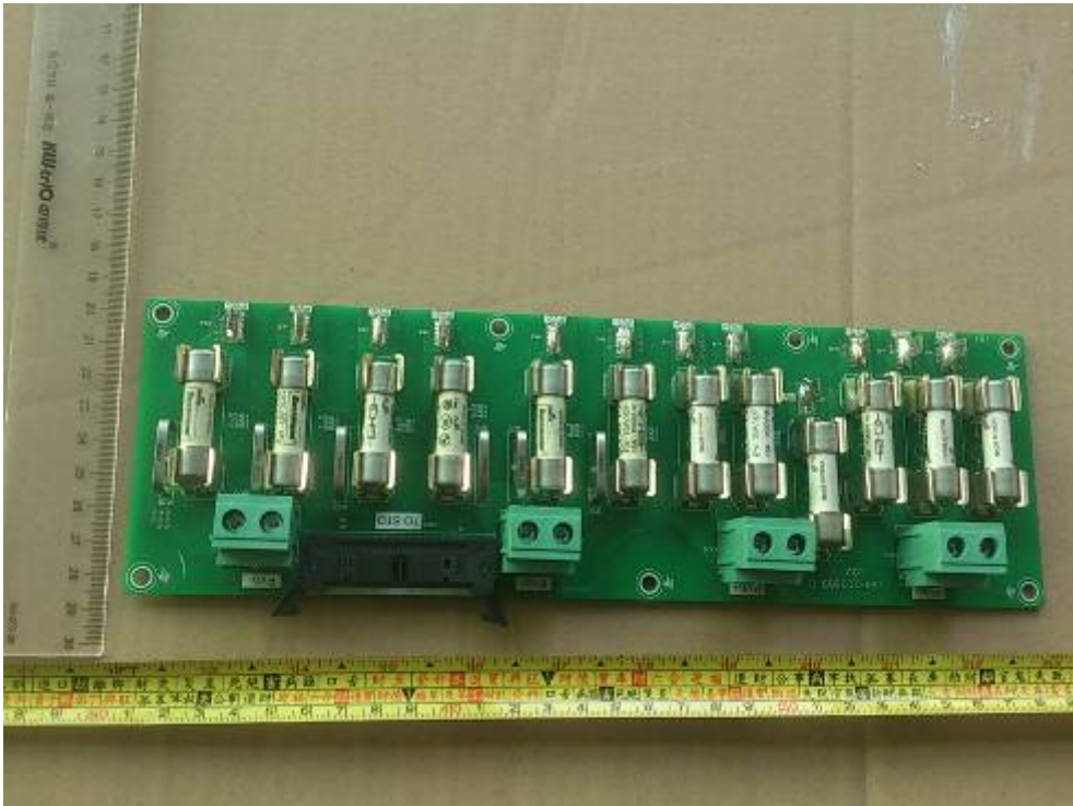
Front view of the fuse board
